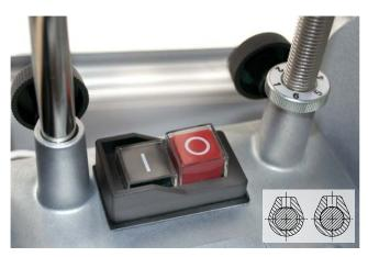
With the sleeves for the Universal Support now being cast in the zinc top, together with the new Tormek stadium shaped design of the holes (patent pending) - the precision have been improved significantly. It will improve your control of the sharpening - and your result.
